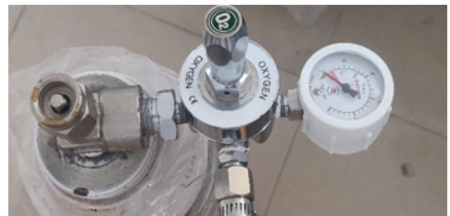
Fig. 1: FA valve with a flow meter that can be directly connected to a patient.
