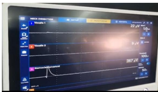
Figure 4: Showing electromyography monitor. In case of critical nerve dissection, it shows an increase in amplitude which alerts the surgeons to avoid nerve injury
